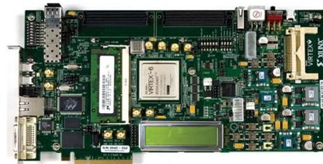
Figure 1: ML605: Xilinx Virtex 6 development board
