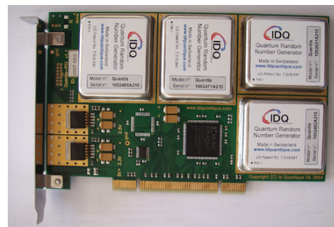
Figure 1: Quantis RNG Card for PCI Bus, showing four independent quantum generator devices.
