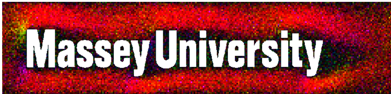
Figure 4: The Lattice Gas Cellular Automata simulating fluid flow past the “Massey University barrier”. The cells are coloured using the HSV colour model with hue defined by the direction of the flow and the brightness determined by the velocity.
