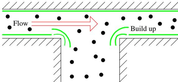
Figure 1: Animat flow at a T-Junction. What will be deposition/scale build-up behaviour and can we engineer animats to de-scale the walls of an artery or other pipeline system?
